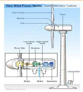
Fig. 1 Horizontal axis Turbine
